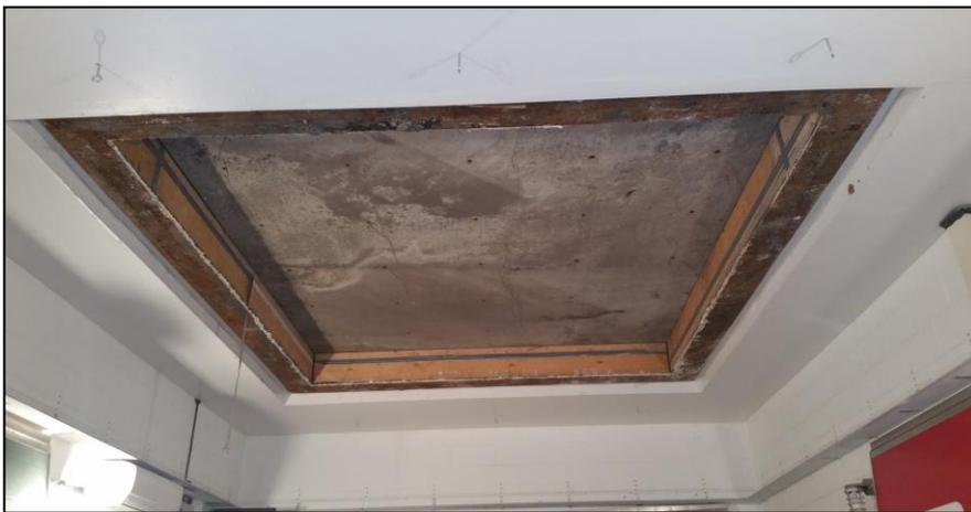
**Receive Room View of Test Specimen Installation**
